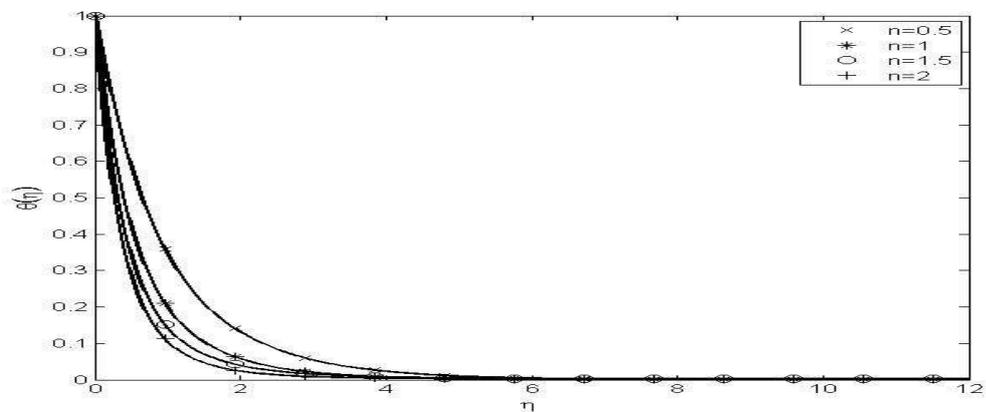
Figure 9: Temperature distribution versus  $\eta$  when  $Pr = 7, S = 0.5, M = 0.5, \beta = 0.5, \delta = 0.5$ .
