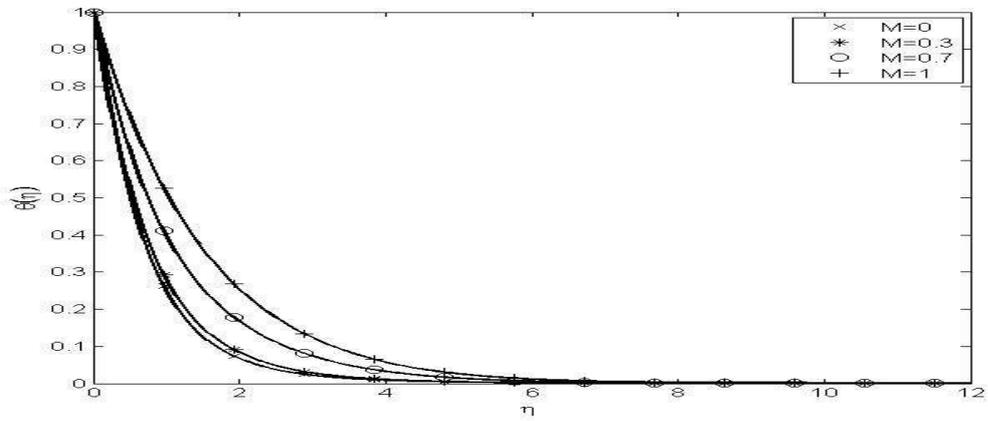
Figure 4: Temperature distribution versus  $\eta$  when  $Pr = 7, S = 0.5, n = 0.5, \beta = 0.5, \delta = 0.5$ .
