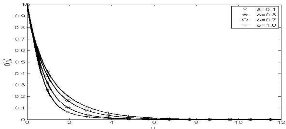
Figure 6: Temperature distribution versus  $\eta$  when  $Pr = 7, S = 0.5, M = 0.5, n = 0.5, \beta = 0.5$ .
