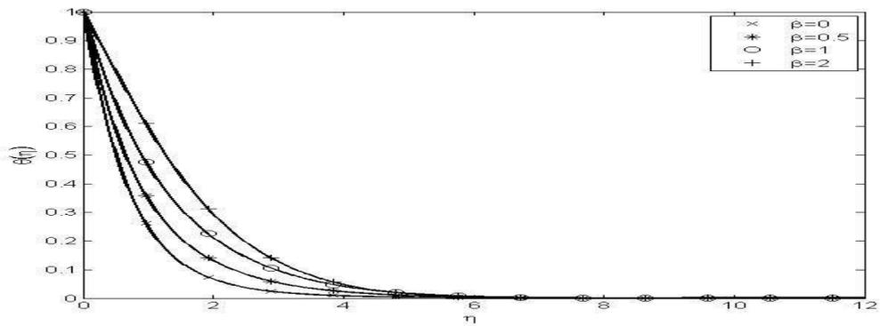
Figure 5: Temperature distribution versus  $\eta$  when  $Pr = 7, S = 0.5, M = 0.5, n = 0.5, \delta = 0.5$ .
