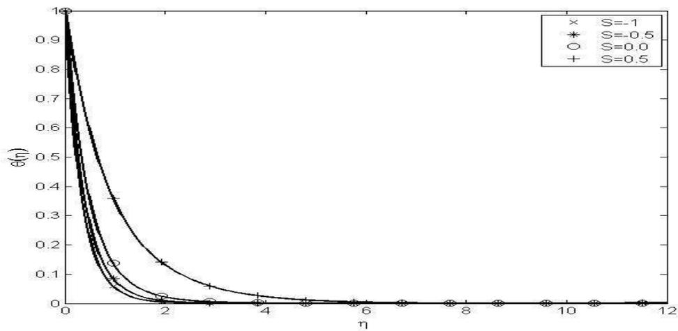
Figure 8: Temperature distribution versus  $\eta$  when  $Pr = 7, M = 0.5, n = 0.5, \beta = 0.5, \delta = 0.5$ .
