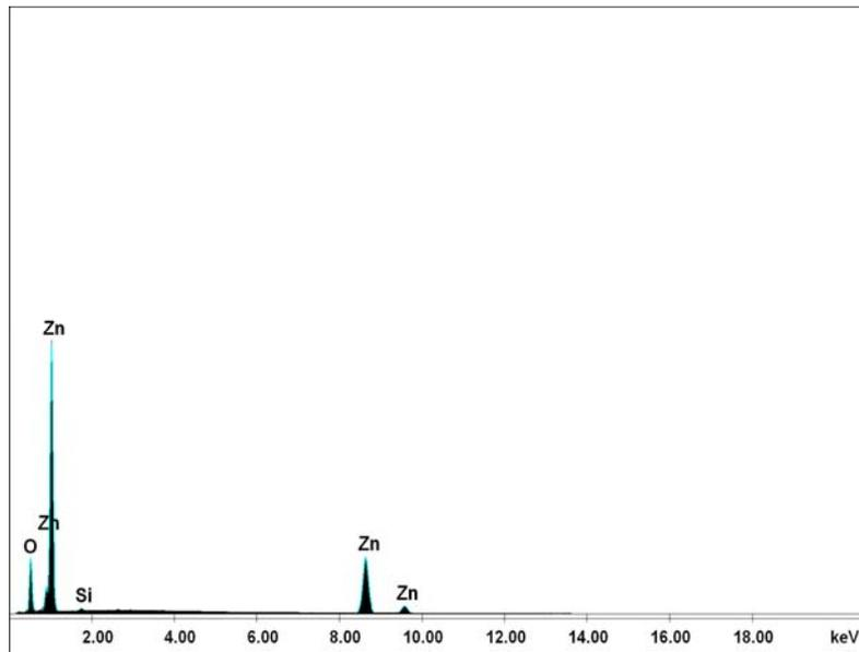
**Figure 10.** EDX spectrum of ZnO
