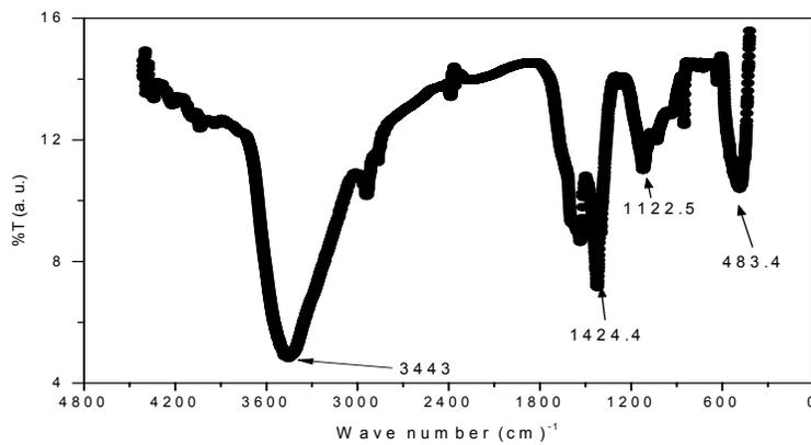
**Figure 11.** FTIR spectrum of ZnO
