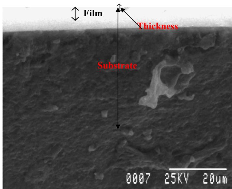
**Figure 1.** Cross-sectional SEM of ZnO film
