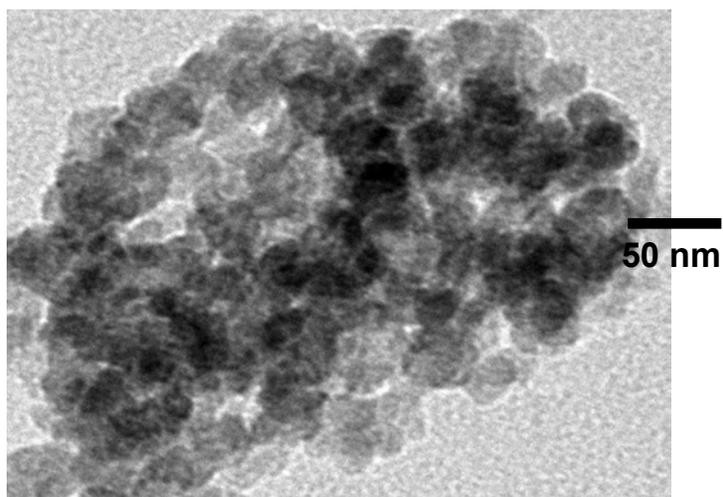
**Figure 6.** TEM image of ZnO prepared from ammonium zinacte bath
