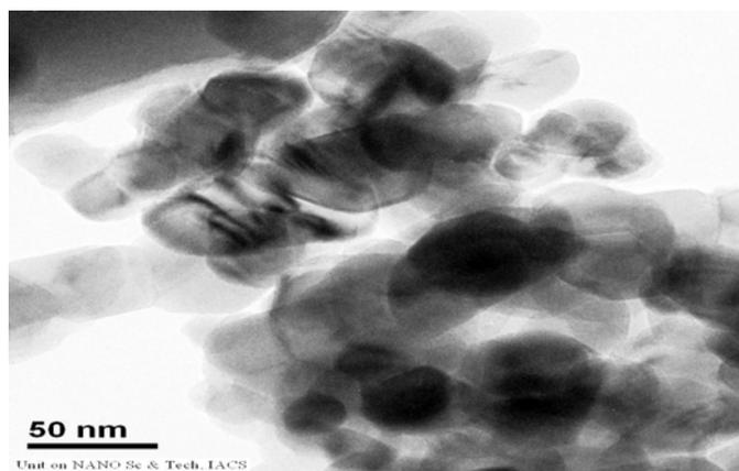
**Figure 9.** TEM image of ZnO prepared from sodium zincate complex
