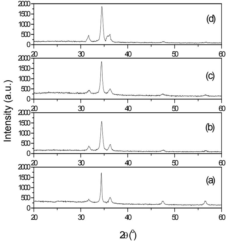
**Figure 2.** X-ray diffraction pattern of ZnO thin films heat treated at (a) 200°C, (b) 300°C, (c) 350°C and (d) 400°C
