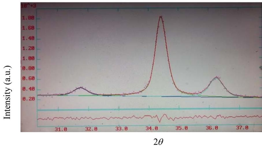
**Figure 4.** Observed (dotted) and simulated (continuous) XRD patterns of ZnO thin film heated at 350°C
