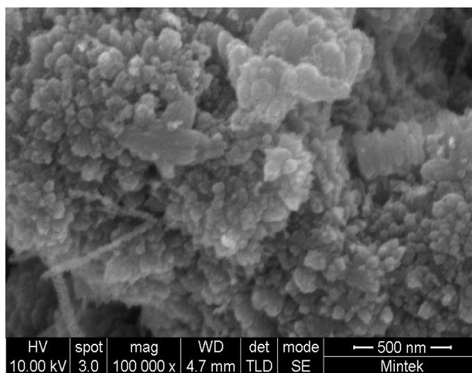
**Figure 7.** HRSEM image of ZnO prepared from zinc chloride precursor
