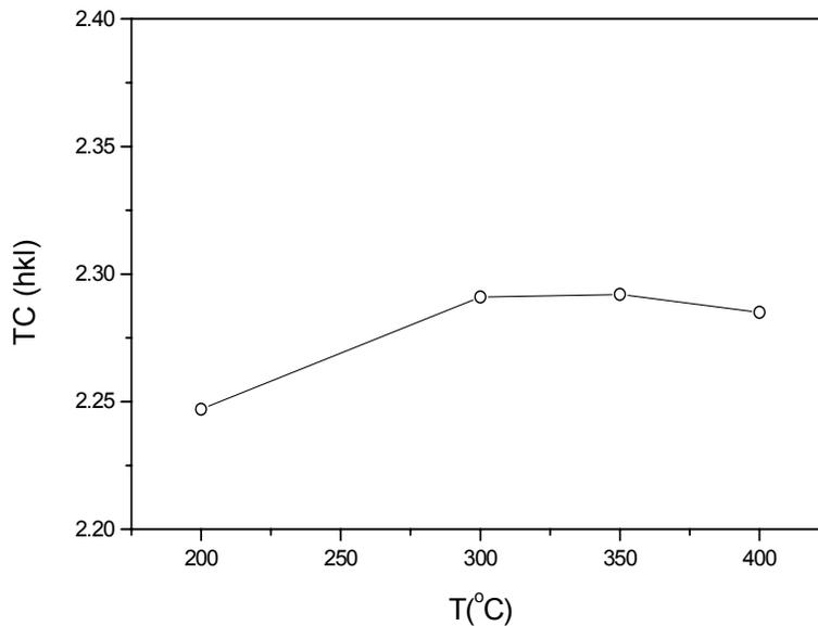
**Figure 3.** Variation of TC(hkl) values of the (002) peak of ZnO films with temperature
