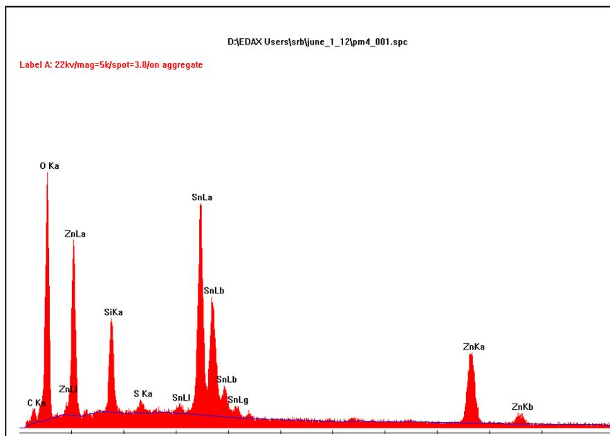
Figure 4. EDX spectrum of Sn:ZnS
