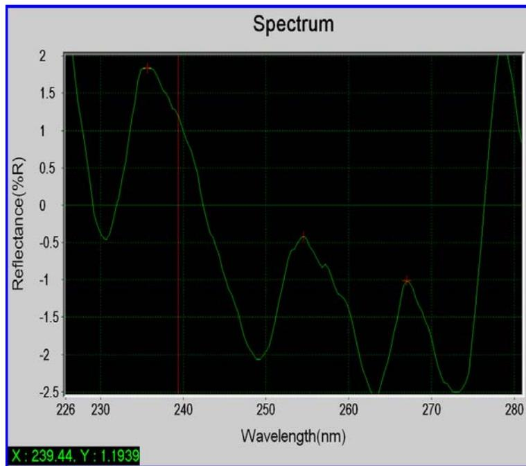
Figure 1. Reflectance pattern of Sn:ZnS thin film
