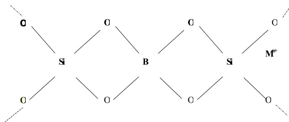
Figure 1. Borosilicate network
