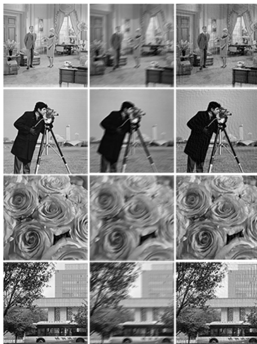
(a) Original image (b) Blurred image (c) Restore image Figure 4: Restoration result of motion blurred image
