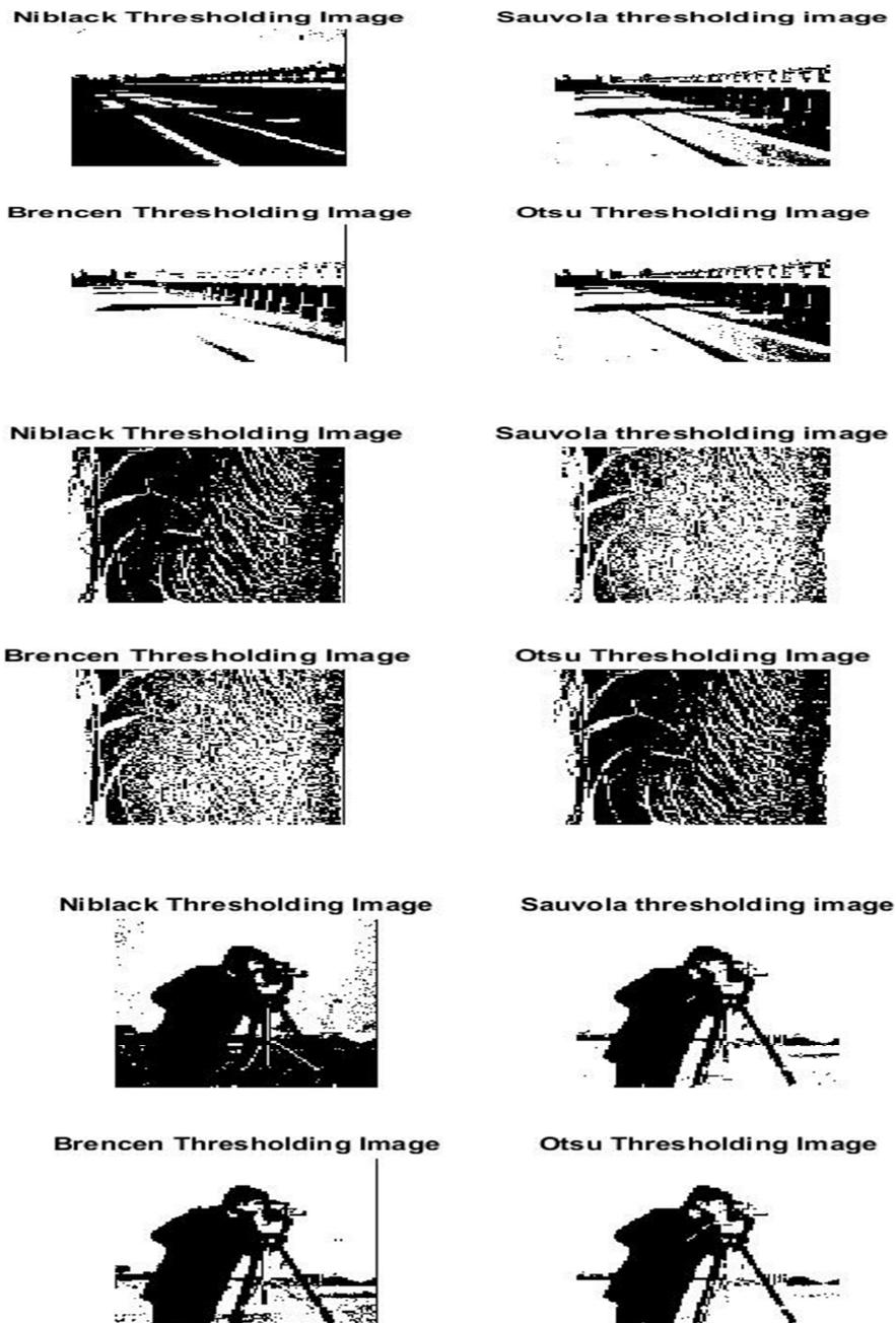
**Figure 4:** The images obtained from the threshold technique methods after performing an initial treatment on the blurry images
